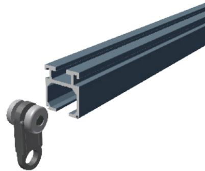
Northgate's 2 Way Track is a medium duty system designed for walkalong use such as side masking curtains, perimeter tracks in studios, acoustic curtains or any other application where walk along operation is required. It is intended for systems where cording isn't required. The 2 way track can be rolled to any radius, the min being 750mm and is stocked in lengths of 6.1m. The external dimensions of the 2 Way track are 35mm (1 3/8") wide x 40mm (1 5/16") high.
