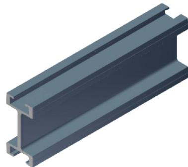
The Northgate Unibeam is an aluminium extruded anodised track section. The standard stocked length for Unibeam is 6.1m and is rigid enough to be used as a suspension beam. It can be pre-rolled to a minimum radius of 2m and the symmetrical design allows it to be used either way up. With the addition of the Trackdrive motor it can become a fully motorised system.
